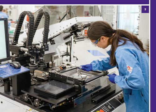
Thinking big about small materials, researchers in Northwestern Engineering's Materials Innovation Lab are advancing additive manufacturing at the nanoscale, developing methods to produce sustainable materials and inks that will help build the biosensors, batteries, transistors, and neuromorphic devices of the future.
